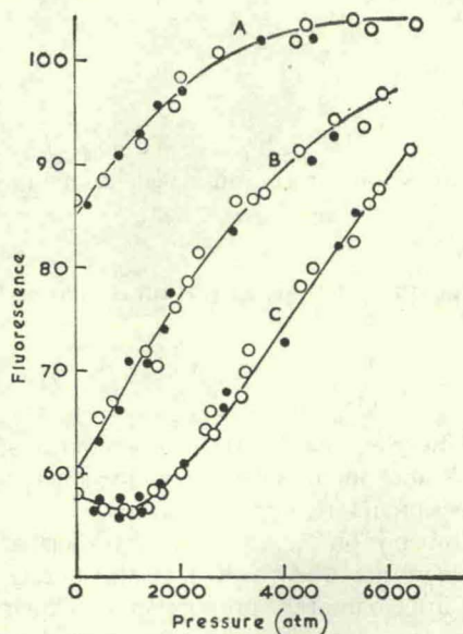
FIGURE 3. (A) 9,10-Diphenylanthracene ( 5 \times 10^{-5}M ) in toluene at 20^\circ . (B) Oxygen ( 7 \times 10^{-3}M ) present. (C) Carbon tetrachloride ( 0.13M ) present
